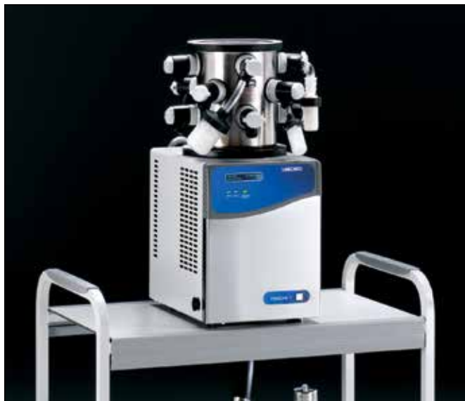
FreeZone 1 Liter Benchtop Freeze Dry System 7740020, 12-Port Drying Chamber 7522800, Portable Table 8025000 and miscellaneous glassware.
